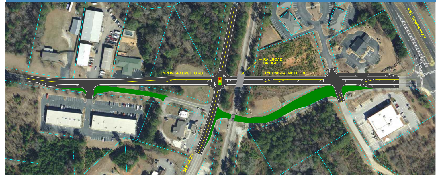
Graphic 4.7 - Concept: Grade Separation at Railroad and Roundabout
